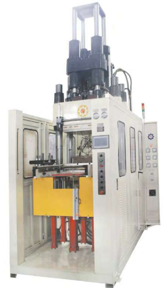
全自动先进先出射出成型机 Fully automatic FIFO injection molding machine (First in,First out)
