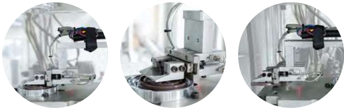
◀ 配备机械抓手, 全自动抓取产品 Equipped with a mechanical gripper, fully automatic grabbing of products
