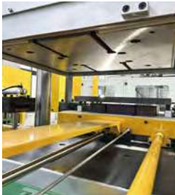
夹板前进, 强制分离模具与上热盘 Lock pin moves in, automatically separate mold from upper platen.
