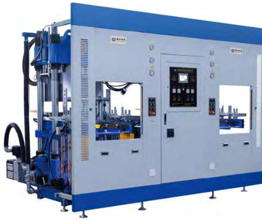
全自动真空平板硫化机(CE) Full-Automatic Vacuum Plate Vulcanizing Machine (CE)
